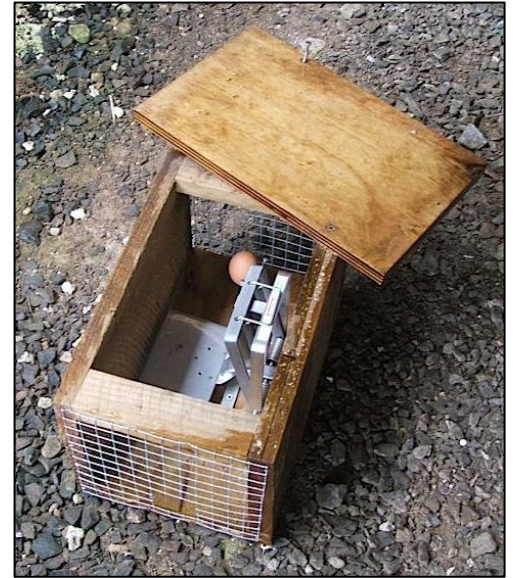
A DOC200 trap with an egg as a lure.
