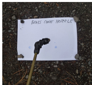
Backpack Sprayer Use a long brass wand and brass cone nozzle and anti drip filter
