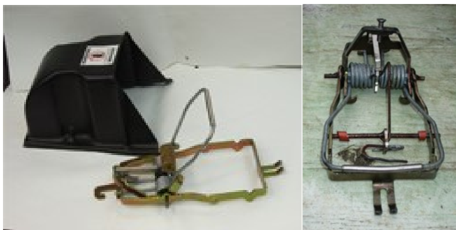
Figure 14. Trap (trigger set in position for possums) and possum cover (left). Trap with trigger in position for ferrets (right)
