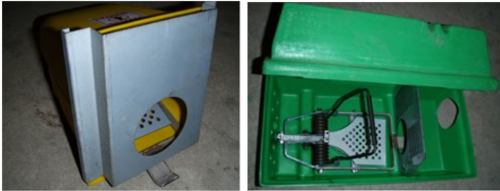
Figure 16. Ferret trap sets with a) the face-plate and yellow trap cover and b) Trappers cover. Note the footplate that is used to trigger the trap when targeting ferrets.
